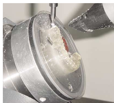
Fig 6. Automated aligner cutter.
