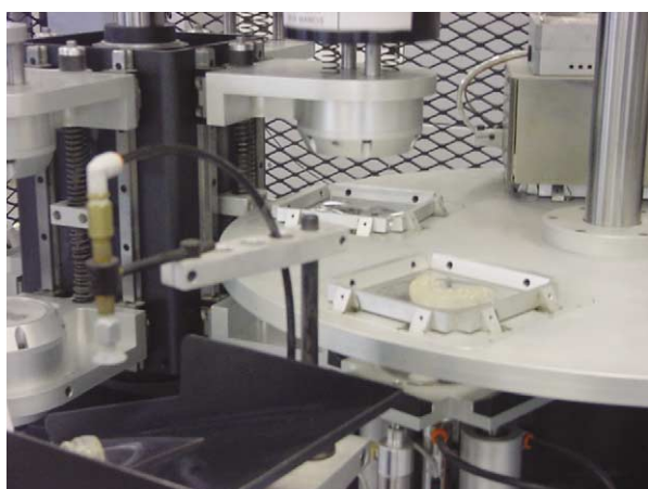
Fig 4. Automated aligner former.
